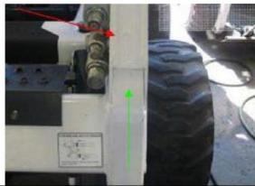
This illustration highlights the base of the push arm hydraulic rams (blue arrows), the countersunk pivot points (green arrows) and the inlet to the radiator fan (red arrow). All areas must be thoroughly cleaned and inspected.
