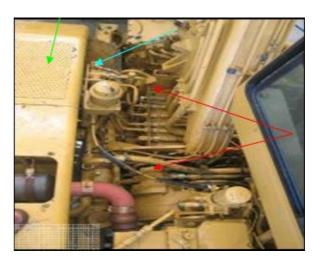
The two chassis rails either side of the engine block are hollow (aqua arrow). On most models there will be access points or drainage holes. The one illustrated in this picture is located on the topside of the chassis rail, towards the rear.
