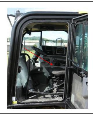
Close up shot of the joystick control panel. Note that access has to be provided to verify internal cleanliness in and around controls. Non affixed panels have been removed (red arrow). Also note that the seat and floor mats have been removed.
