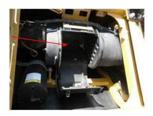
The batteries (red arrow) are to be loosened from the tie-down points and inspected underneath. In newer scrapers the batteries are located under the front of the cab, removing the cover to allow access also allows access to the hollow sections of the front draw bar.
