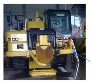
Once the seat has been removed, the internal of the rubber shroud (red arrow) can be easily cleaned and inspected.
