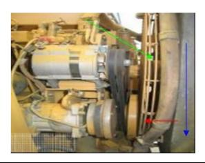
The air-filter is to be removed from the housing (red arrow) and verified clean (usually performed with pressurized air).
