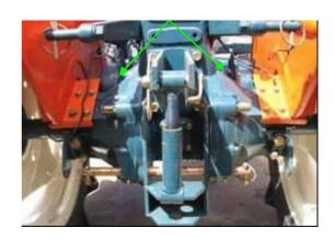
These two illustrations highlight the small recesses that can be found on the rear axles on some models. The green arrows highlight a small gap that must be flushed to verify cleanliness.
