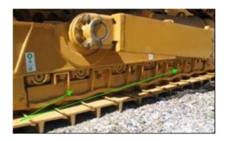
On other small models the topside of the track frame may have numerous non-affixed panels (green arrows) which all must be removed for cleaning and inspection.
