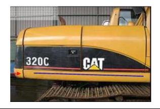
Check all engine doors for hollow support channels. Check for drainage holes or if only spot-welded – will require flushing if not completely sealed. Check all foam insulation and hydraulic hoses (red arrows).
