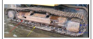
Red arrow indicates that the motor cover has been removed, allowing access to the drive motor. The green arrow indicates the hollow channel, which extends up through the frame into the turret or slew ring. These hollow areas on each side need to be thoroughly flushed to ensure cleanliness. The blue arrow indicates the area at the rear of the motor cover, which can be easily overlooked.
