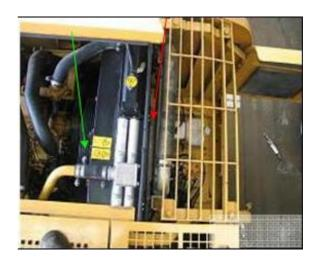
On some models, a mesh grill protects the radiator core. These mesh grills (red arrow) need to be removed as the gauge is small and prevents BRM caught in the radiator fins from being successfully removed.
