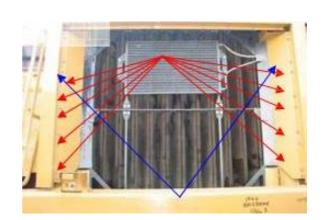
The panels in front of the cabin, which house the air-conditioning and electrics must be removed. All hollow handrail tubing must be flushed in the presence of the inspecting officer. Check all light covers for damage (red arrows).
