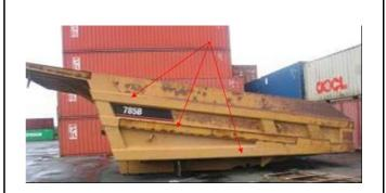
This tray comprises of two segments that are bolted together. Once apart, the ribs along the underside are open and exposed to biosecurity risk material (red arrows).
