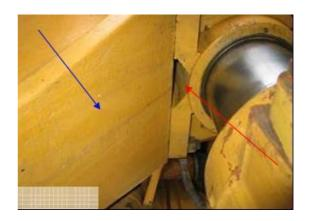
Just right of centre at the rear of the wishbone is a small drainage hole (green arrow). Flushing via the two entrance holes located below either strut will result in water draining from this hole.
