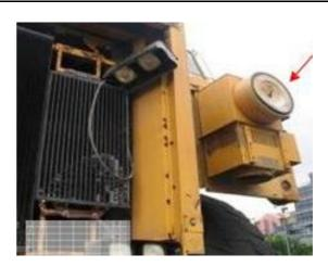
Another example of the front end of a dump truck. This one has an open-ended channel running along the topside of the radiator. To correctly verify if radiator/oil cooling fins are clean, they require flushing from both sides. In this instance, the oil cooling system will need to be removed. This does not require full removal – on some models only a few bolts on one side need to be removed and this front unit can be swung outwards (red arrows).
