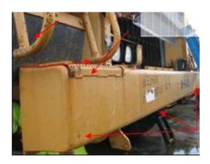
On some models the air-filters are found in a variety of locations. This one is below the cabin and has several hollow channels as highlighted by the red arrow. Filters must be removed and blown with air to verify cleanliness. Have any other non-affixed panels dismantled to allow full access.
