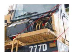
Close ups of the air-conditioning and electrical systems found behind the panels at the front of the cabin. On the left, these tie-down hooks (red arrows) must be loosened off to reveal inside the air-conditioning unit – check filters. The blue arrows in each photo indicate part of the box channel housing of the cabin air-con and electrics inspect in behind this box channel. The use of telescopic or flexible mirrors can facilitate the inspection.
