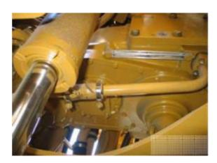
These illustrations highlight the hollow chassis rails (red arrows) and drainage holes (where the belly plate bolts have been removed – blue arrows). The area will require flushing to ensure cleanliness.
