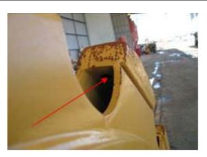
A view of this boot reveals that it is not completely sealed (only spot welded) in place. The green arrow highlights the small recesses, allowing contaminants inside this hollow cavity (blue arrow). These will require further investigation to verify cleanliness. Flushing via these small recesses with a pin jet, will not suffice in removing BRM or verifying internal cleanliness. All boots must be removed (illustrated in second image). Once removed, access is easy for verifying (red arrow).
