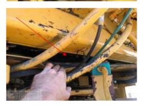
This illustrates the compartment under the cabin step. Like the oil tank on the other side, this area has ledges (red arrow) and hollow channels (blue arrow) that require cleanliness verification.
