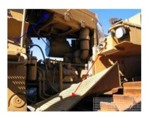
This image shows the side of the engine block (red arrow) and hollow chassis rail (blue arrow). The engine cover has been laid back on the hinge, exposing a small gap (green arrows) between the side cover and the chassis rail. Flush along this small opening to remove all BRM. Flush checker plate (aqua arrow).
