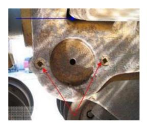
On the ends of some models will be protective plates (red arrow). The structures are generally hollow and need to be flushed via the small open gaps at the bottom (blue arrows) to ensure cleanliness.
