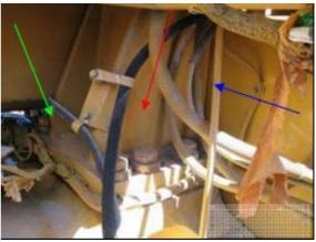
This image shows the hollow channels located just below the floor pan. The red arrow indicates where the opening can be found. These channels require flushing to verify cleanliness.
