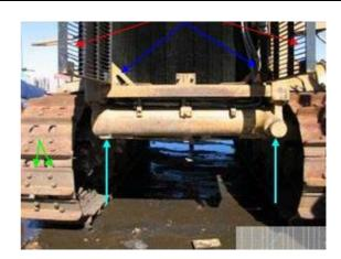
The green arrow highlights the hollow vertical pillars either side of the radiator. Flush in the presence of the inspecting officer if these are not sealed. Check for any ledges or open-ended channels as above the radiator core (red arrow). In this instance, the circular nose bar is hollow and can be accessed for flushing via the belly plate bolt holes (see aqua arrow and the following image). All radiators must be flushed in the presence of the inspecting officer to verify cleanliness.
