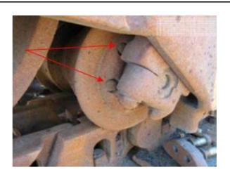
The track guides have been removed for ease of cleaning and inspection. On some models the two bolt ends (red arrows) are countersunk at the rear of the track guide. Ensure that the rear of this guide is checked for any biosecurity risk material (BRM) in these areas (blue arrow).
